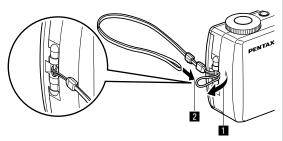
Pass the narrow end of the strap through the strap lug and pass the other end through the loop.
